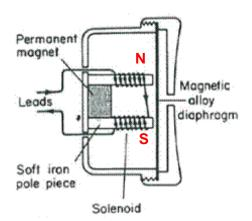
The telephone receiver contains a U-shaped magnet formed by placing a short permanent bar magnet across the ends of two soft-iron bars (Fig. 36.14). This is placed so that it exerts a pull on a springy magnetic alloy diaphragm. Two solenoids are wound in opposite directions on the soft-iron bars.
